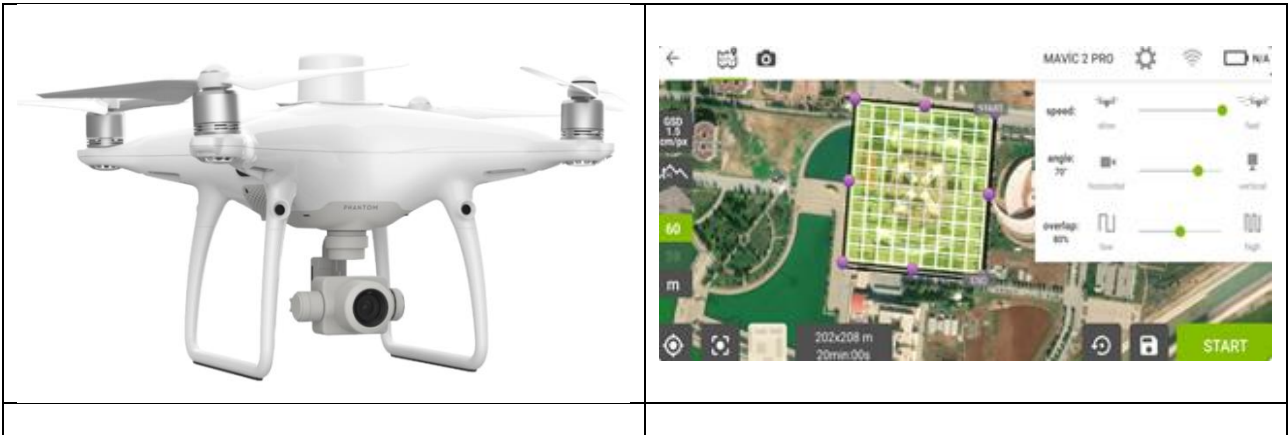
Figure 1: DJI ENTERPRISE PHANTOM 4 RTK UAV used for this flight mission and flight plan example
