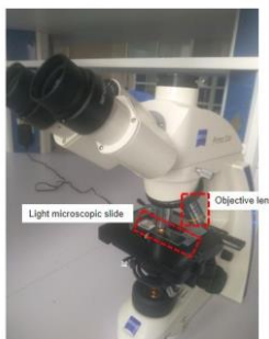
Figure 1. Light microscope with a trachea slide
